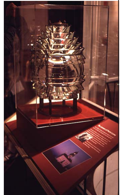
The fifth order Fresnel lens (above) on display at "The Lighthouses of Point Loma Exhibit" is a smaller version of the large third order lens shown in the design sketch below. (NPS photo by Paul Koehler)
