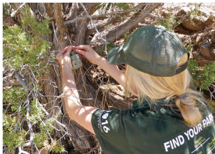
Hanging the air-temperature sensor.
