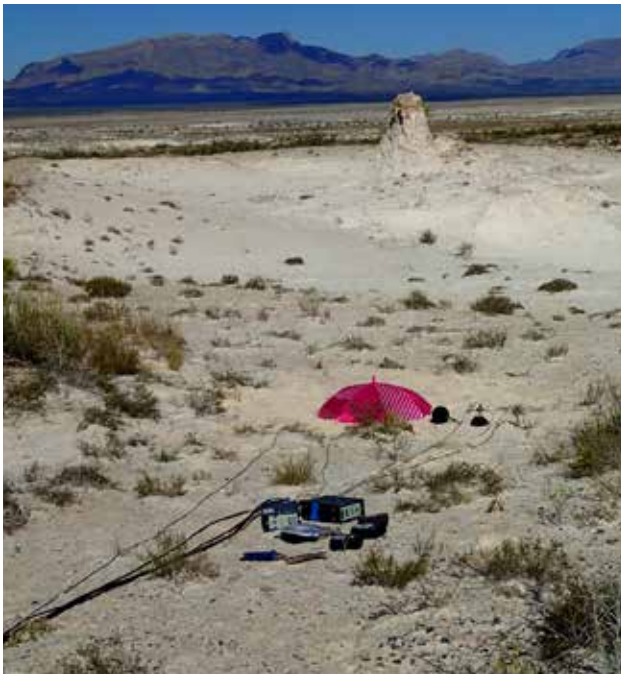
Figure 1 - Microphones and miscellaneous equipment at NE30—the sonic boom testing site.
