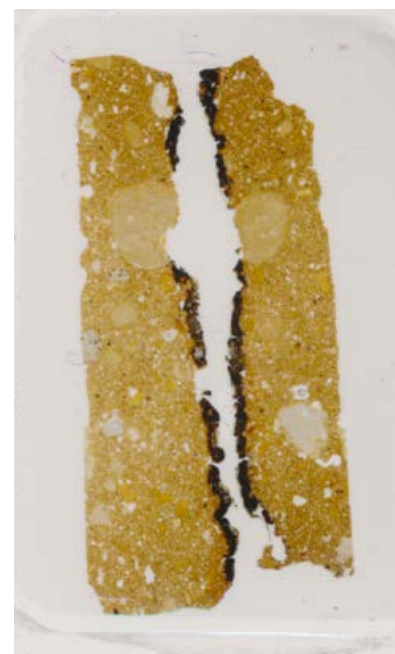
Figure 4. SEM thin section of plaster from the Room 21 exterior wall. The dark line is soot and dust that accumulated on the wall surface over time. (Source: Bass et al. 2015:8).
