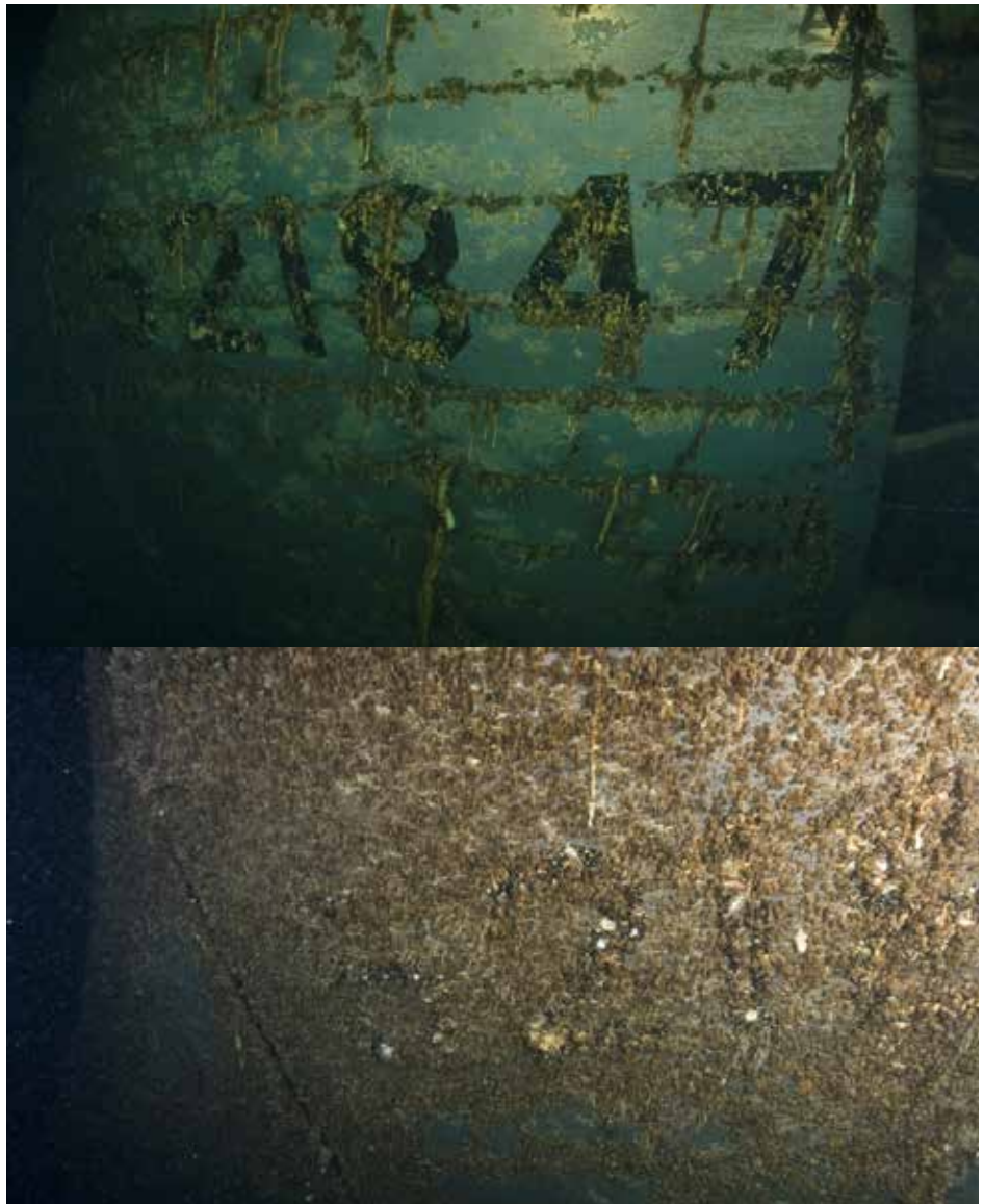
Figures 10 and 11. Before and after: an example of quagga mussel fouling on the B-29 at Lake Mead National Recreation Area from 2006 to 2009. NPS Submerged Resources Center Archives.
