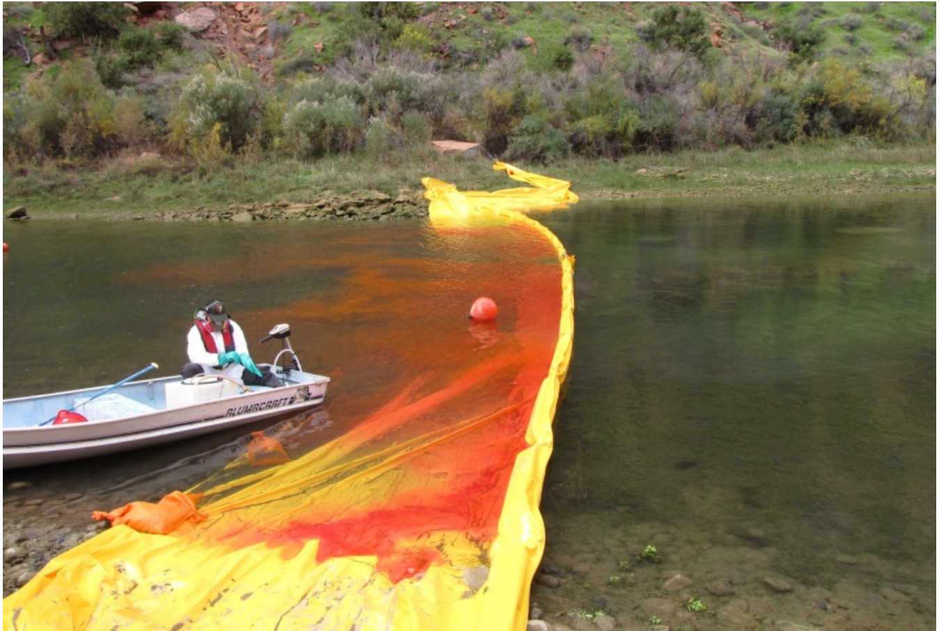
Figure 6. Impermeable barrier prevented test dye and piscicide applied inside the slough (left) from mixing with main river flow (right) (Melissa Trammell, NPS).
