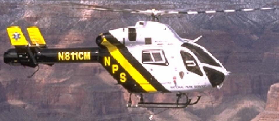
**Grand Canyon National Park is reducing noise from NPS aviation use by flying an MD-900 Explorer NOTAR (No Tail Rotor) helicopter for park operations. In addition, area tour operators are joining NPS efforts to implement quiet technology and restore natural quiet.**
