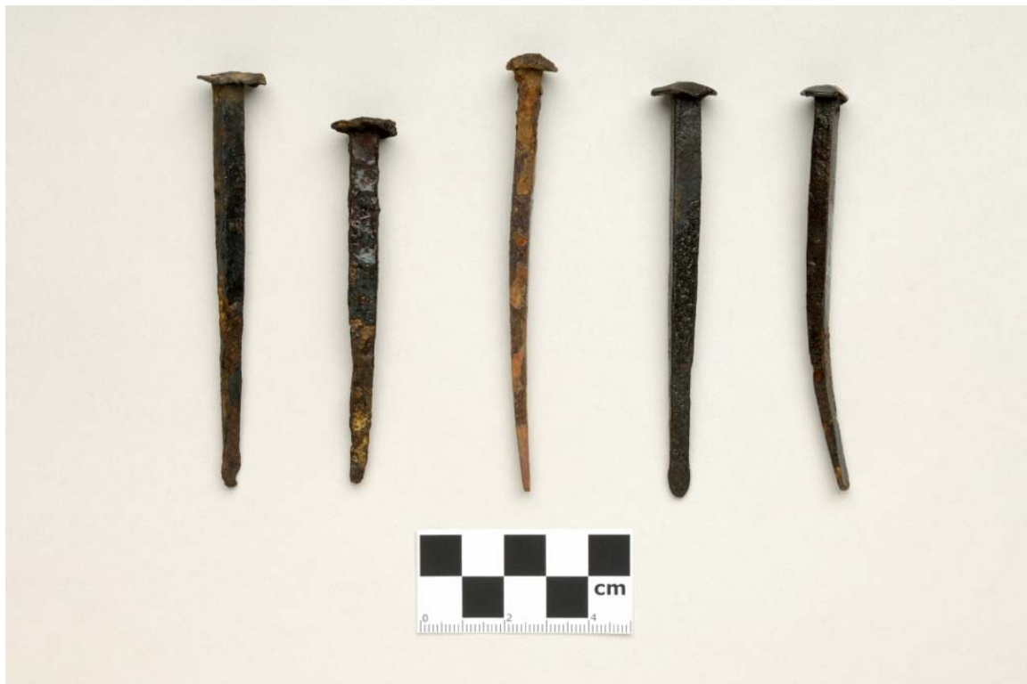
Photo 28. A sample of nails from the SARA-00387. All hand-wrought, both "T-headed" nails and roseheads. All appear to be burned and annealed.
