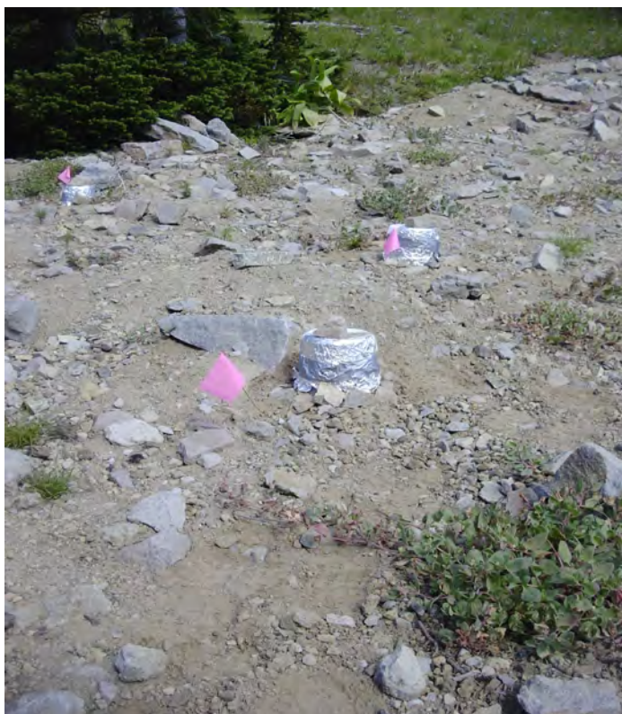
Figure 4: Photograph of Carbon Dioxide Detection by Soda Lime Absorption
