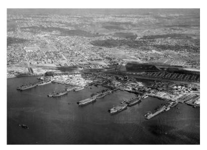
2. 7. US Navy Repair Base, San Diego. Between 1943 and 1945 the base performed conversion, overhaul, maintenance, and battle damage repair to more than 5,117 ships. Central to this maintenance were the Navy's construction and delivery of 155 new floating dry docks deployed to various bases, including three 3,000-ton, three 1,000-ton, and one 900-ton floating docks remaining at the San Diego Repair Base.
