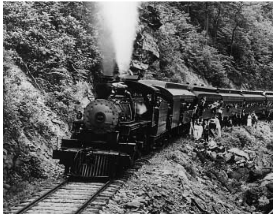
Early tourists and sightseers on the Little River Railroad. This is a Compound Baldwin Mallet pulling the Elkmont Special excursion around the Little River Gorge (circa 1909–1914).
