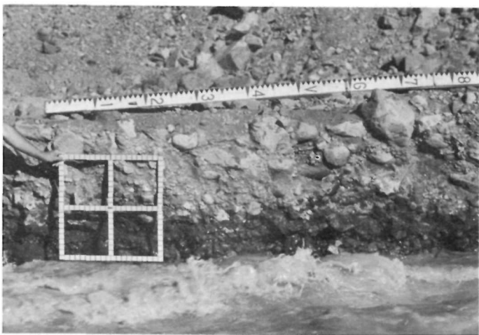
FIGURE 20.—Cutbank in valley train. Note concentration of fine debris at surface. Vertical bank is due to stream erosion of materials with apparent cohesion.
