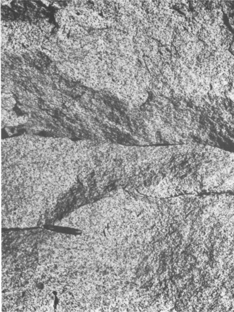
GRANODIORITE looks like granite and has a light-gray speckled appearance. The knife is about 3 inches long. (Fig. 3)
