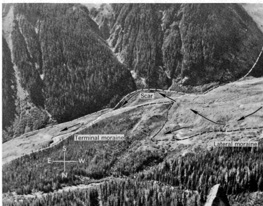
FIGURE 9.—Avalanche scar, about 140 feet high, at the base of Goat Island Mountain. This scar was formed when part of avalanche unit 3 moved through the narrow gap in the terminal moraine (fig. 2). The avalanche deposit downstream (left) from the scar has been partly eroded by the White River. Area of avalanche deposits is enclosed by dashed line; arrows show inferred direction of movement of avalanche unit 3.
