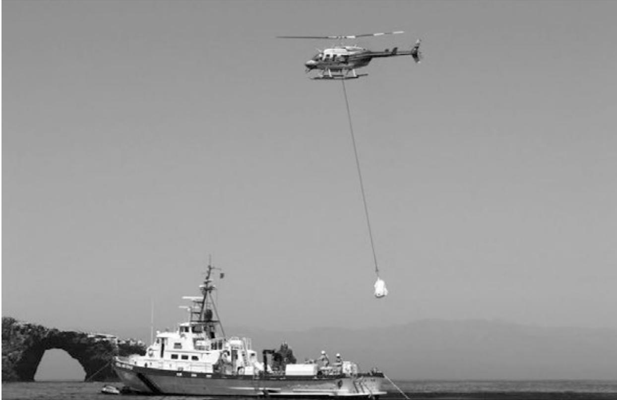
Figure 5-10. For some heavy equipment, including Conex boxes, only helicopters could move them to and from the islands. Here a helicopter is transferring materials from the *Ocean Ranger* to Anacapa Island.
