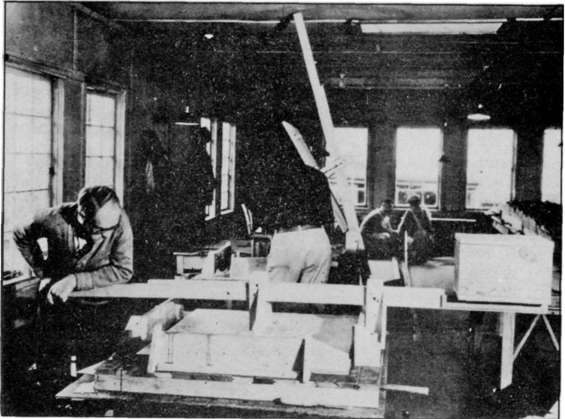
Gluing Down Contour Laminations. This is an improvised press made for the purpose with a 2 x 4 set in supports so that it can be weighted as much as desired. Care should be taken to distribute the pressure over the entire area of the laminations being glued.
