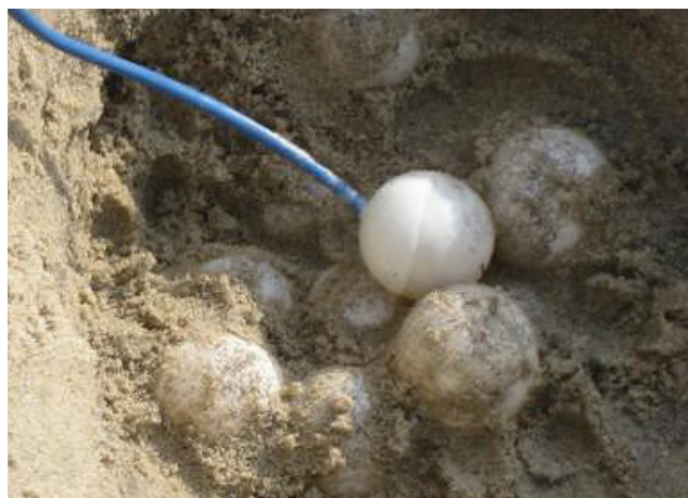
Nest sensor in a sea turtle nest, Cape Hatteras National Seashore. NPS
