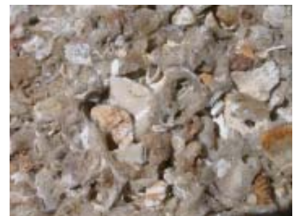
Closeup of coquina from the Anastasia Formation used in the construction of Castillo de San Marcos showing the fragments of fossil shells.
