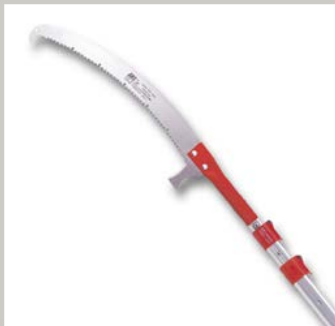
A curved saw blade attached to an aluminum telescoping pole. This blade design includes a back cutter at the base of the saw. A back cutter helps prevent bark from tearing during sawing ( ARS ).
