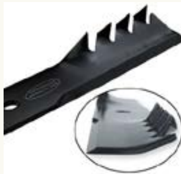
Teeth on the Gator blade direct air flow under the deck so leaf pieces are chopped up more than once ( Green Dealer ).
