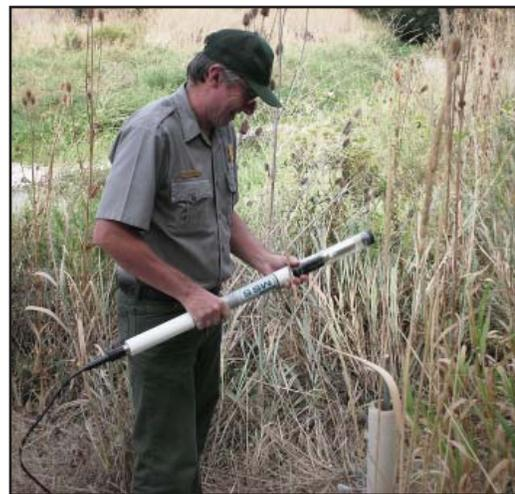
Roger Trick, calibrating the water quality monitoring instrument by Mill Creek, WHMI.
