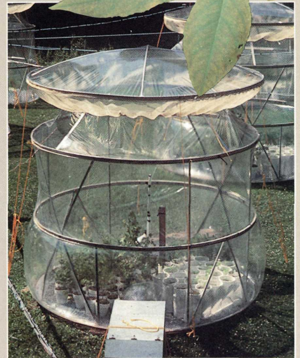
Exposure chambers for testing responses to acid deposition and ozone.
